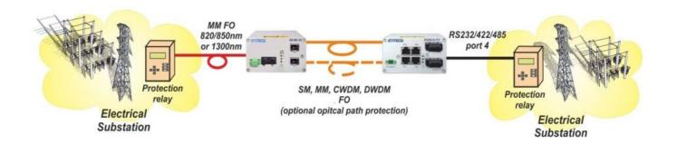
The **BS-MC-50** is supplied with direct current source, with rated voltage value within the range of 12-60V or from an external direct voltage power supply unit delivered on an order by the producer. Device can be mounted directly on the DIN rail.
