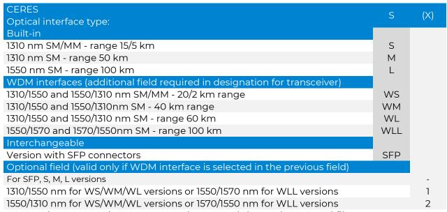
**NOTE** - the ranges given are approximate and depend on actual fibre parameters
